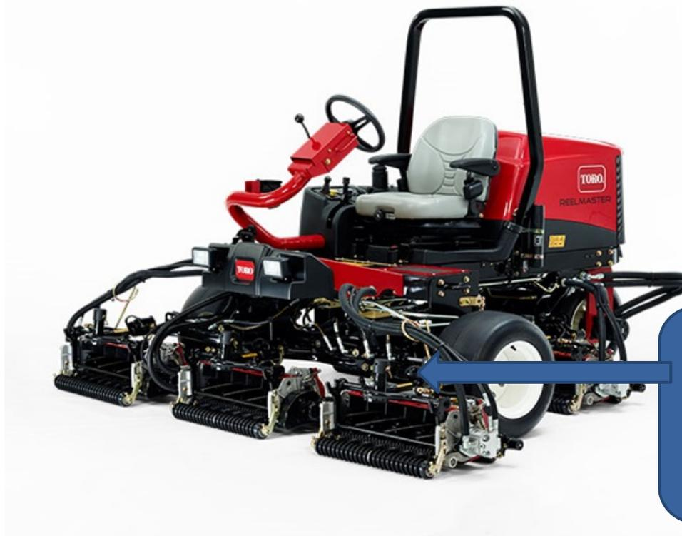
The cutting units are taller with vertical fins promoting clipping ejection or not bogging down the unit giving a great cut the first time.
