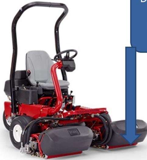
Damage is minimized from the blades being pulled by a large front roller instead of pushed like other mowers.
