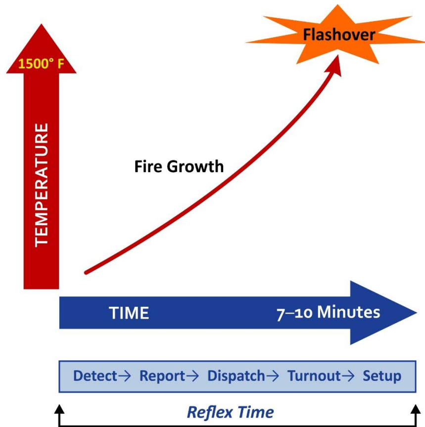
Figure 128: Illustration of Fire Growth & Fire Department Response Time Components
