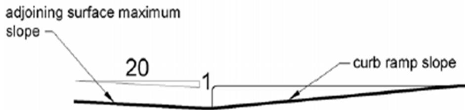
Figure 406.2 Counter Slope of Surfaces Adjacent to Curb Ramps
