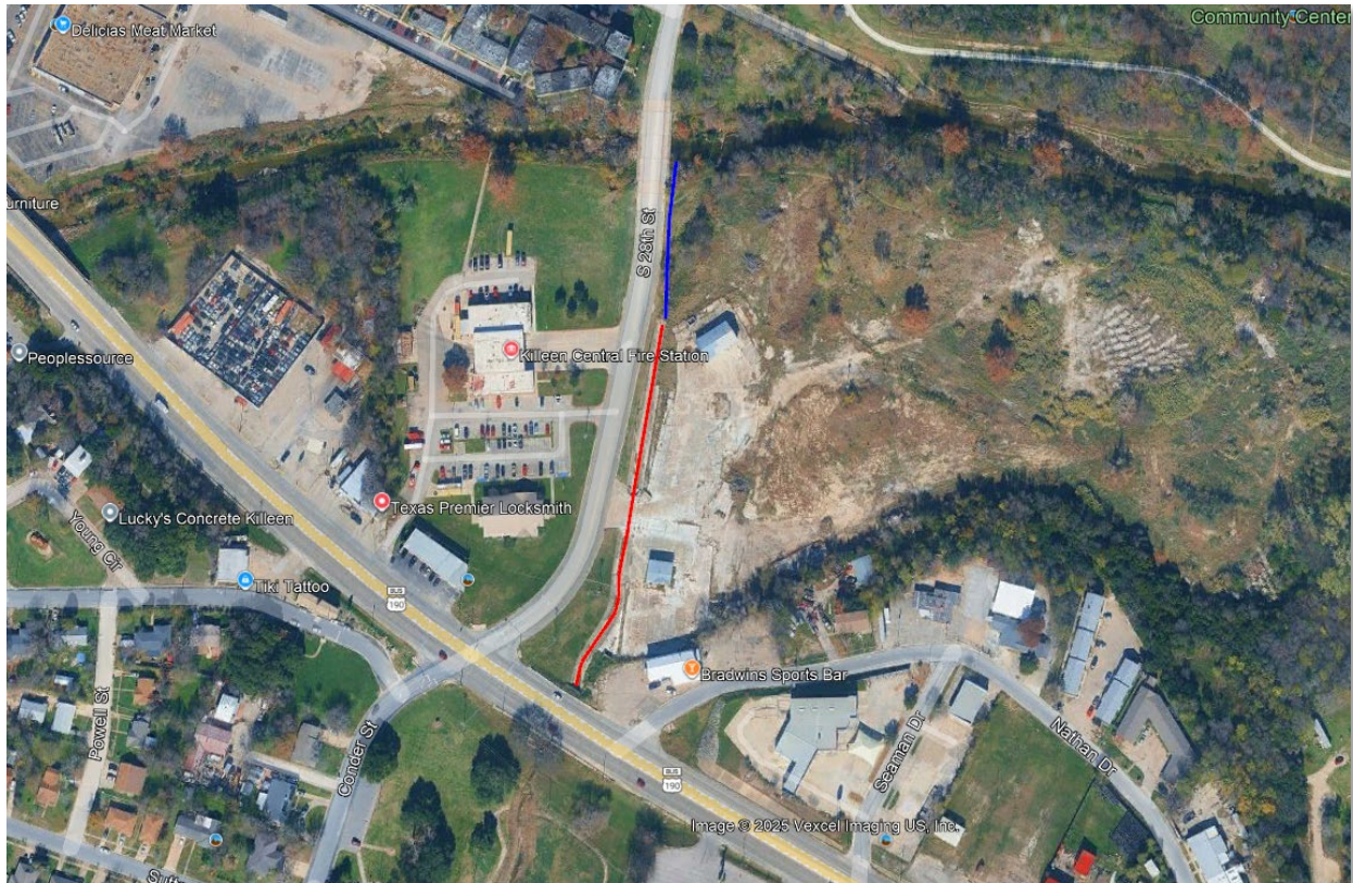
Figure A – Project Area Map (Red is Existing Channel, Blue is Proposed Diversion)
